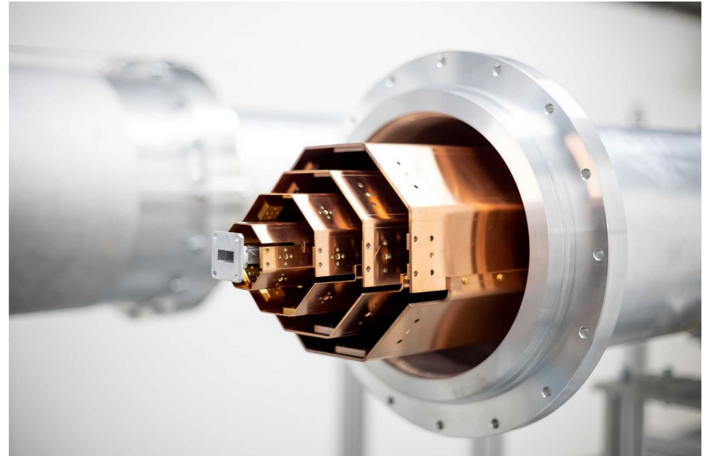
A view inside a section of the 30-metre-long quantum connection. An aluminium waveguide (centre), cooled to almost absolute zero, connects the two quantum circuits. Several layers of copper shielding protect the conductor from thermal radiation.
