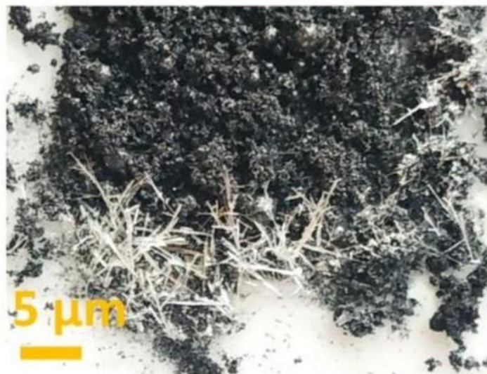
Fig 2: Hair-shaped structures of molybdenene (right) are formed in the microwave (left). Copyright: Sahu, T.K., Kumar, N., Chahal, S. et al, Nat. Nanotechnol. (2023)
